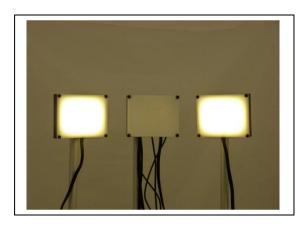
Different patterns of on/off and brightness can be used. Master boards can be used individually as well as in combination with Clients. Each Master can support up to two clients.
