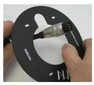
Then align the plate on the surface of the HC-MIS so that the fours screws can be inserted.
