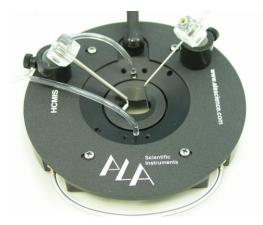
The HC-MIS can be fitted with an optional plate to allow the use of magnetic tools which cannot adhere to the aluminum frame of the HC-MIS.
