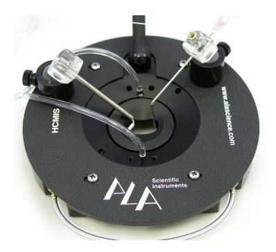
HC-MIS: shown at left with optional magnetic plate and magnetic swivel tools from ALA (MU-TOOL holding a thermistor sensor, and stainless steel perfusion canula). Also shown are gas input ports and tubing. At lower end part of the cooling fluid loop tubing is visible.
