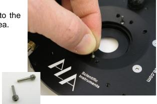
1.5mm tubing can be slipped over the stainless steel tubes, and a 'Y' connector makes an easy hook-up to a gas supply.
