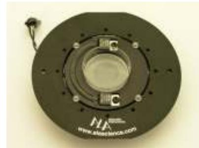
The *HCS* has a steel outer ring allowing for magnetic tools to be used. The inner ring contains the heater and feedback sensor.
