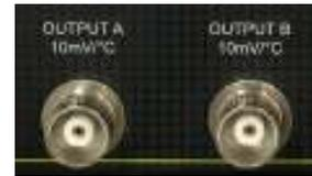
Each 10mV output corresponds to a 1°C temperature reading. For example, a *SENSOR A* temperature reading of 45°C translates to a 0.45V (450mV) output.
