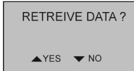
Use the UP/DOWN buttons on the front panel to select YES or NO. On the first time powering up the HCT-10 there is no data stored other than the default values.
