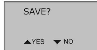
Continue scrolling if to continue using the current parameters without saving them or press the DOWN button. Press the UP button to save the parameters for future use. Any changes made after this screen will have to be saved prior to turning the HCT-10 off.
