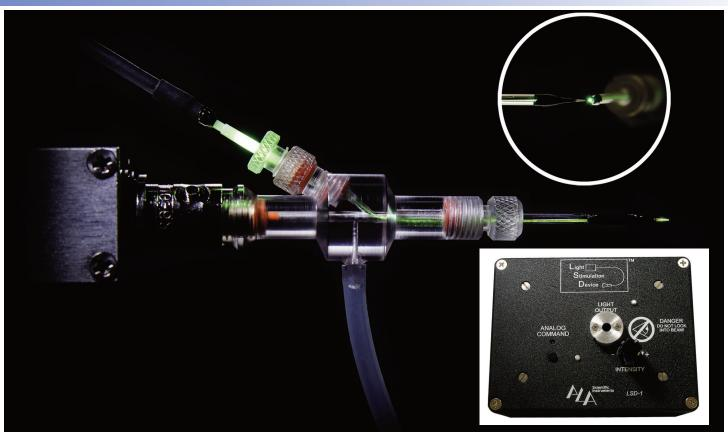
The Optopatcher is a new micropipette holder with integrated optical fiber to allow simultaneous patch-clamp recording and optogenetic activation. The design eliminates the need for a separate manipulator for optical stimulation. When combined with ALA's **LSD Light Stimulator Device** a complete ecomonical optogenetics system is formed.
