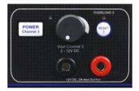
demand will need to be cleared or the channel will continue to alarm. The polarity of the output is shown by the colors of the banana plugs for the output. Red is positive (+) and black is negative (-). Polarity cannot be reversed internally.
