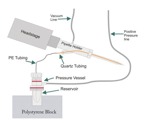
The above diagram shows the system used with the quartz tube in its original size (not prepared). The quartz tube has a 100um id and will allow for higher flow rates when used in this manner. However, this also impedes the quartz tube from getting close to the cell as the pipette narrows at the end. Being closer to the cell increases the response rate.
