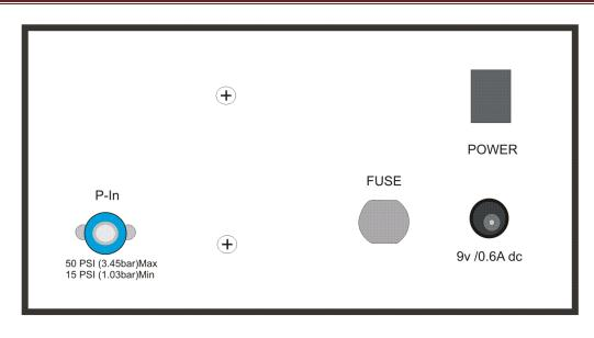
The rear panel of the 2PK+ Pressure/Vacuum Generator has 2 connections.
