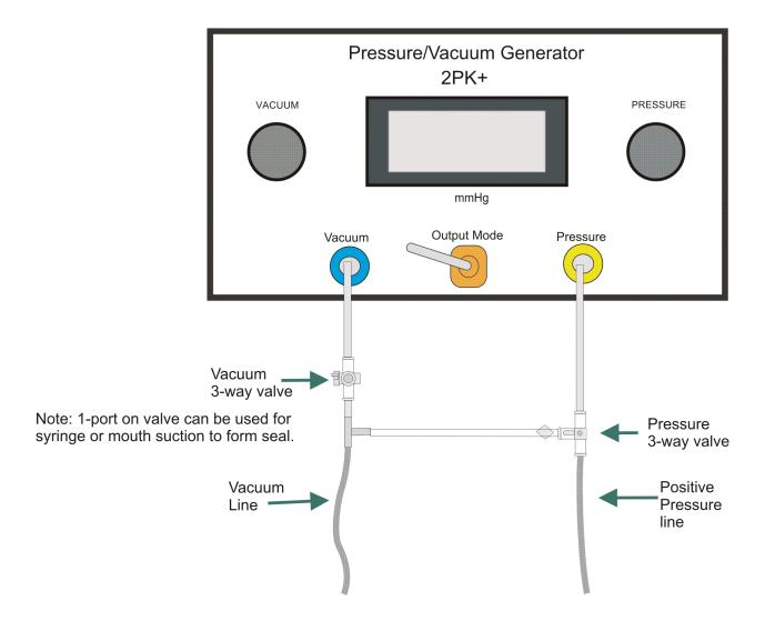
The tubing and luer valve assembly must be connected to the front of the pressure/vacuum generator (PVG). Connect the assembly as shown in the above diagram.
