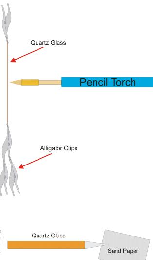
of scissors, wire cutters or other implements. The final tip size should be no less than 35µm. Larger sizes can be experimented with. With the advent of the positive pressure vessel, it may be possible to perfuse without pulling the quartz capillary. However the small size of the tip will help place it further down into the pipette tip. It should not be necessary to make a fresh quartz capillary for each experiment. One capillary should last through several experiments before requiring a change.
