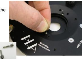
1.5mm tubing can be slipped over the stainless steel tubes, and a 'Y' connector makes an easy hook-up to a gas supply.
