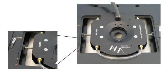
The HC-MIS is simply dropped in and the two screws with cap heads are backed out until it fits snuggly in the center of the square hole.
