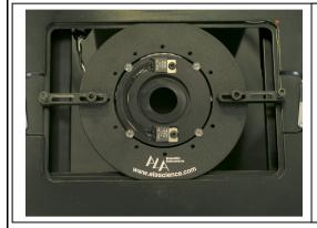
Mounting system for **Zeiss K** stage. Two armatures are attached to stabilize the HCS in the K frame opening.
