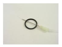
Pierce the o-ring with a 19GA needle, insert PE-10 tubing through needle.
