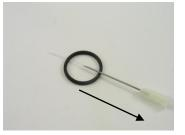
Withdraw needle so that tubing remains passing through O-ring.
