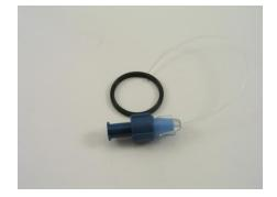
Withdraw PE-10 tube until end is just inside o-ring. Place Luer compression fitting on tube. Additional holes or cuts can be made in o-ring to facilitate fluid evacuation from the chamber. Short lengths of tubing may be used as outflow ports as well.
