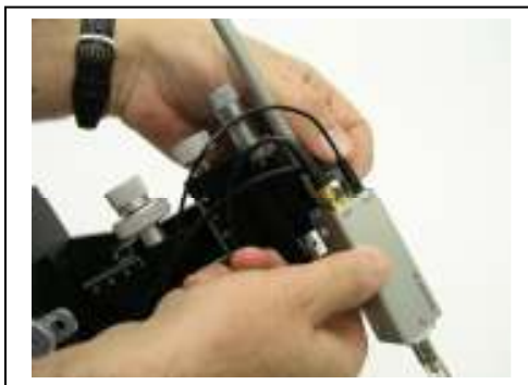
Mount the Potential head stage on the left side, and the Current head stage on the right.
