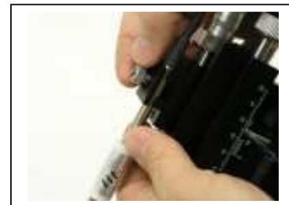
Mount the Potential head stage on the left side, and the Current head stage on the right.
