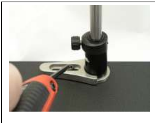
Left side post, adjusting the swivel. Note the locking knob is on the left.
