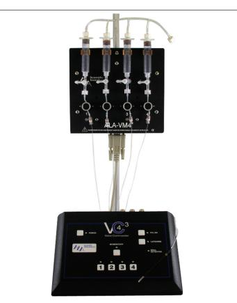
Complete 4-channel pressure driven system with optional compression fittings and QMM Micromanifold®
