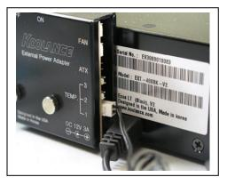
Since CPU coolers are usually powered through the power supply of the computer, this one requires a 12V power adapter with wall transformer. The transformer is universal so it can work anywhere in the world. The power switch is located on top of the power module shown in the photo above.
