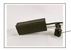
The HCPC can be mounted on a magnetic base with a swivel as pictured above, or via mounting rod ( $3.2mm \ 1/8^{th}$  in.) Rods are about 10cm long.
