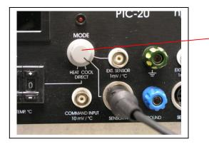
Remember on the npi PTC that when the mode switch is set to Direct, DC Voltage will be supplied to the HCPC. The amount will be set by the pin-wheels. The number you set represents a percentage of the full power that can be applied. The Limiter is by-passed in Direct mode, so for example 500 represents 50% of 14 Volts, or 7 Volts.
