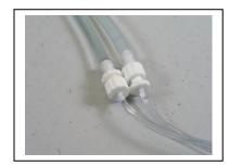
Two Luer fittings shown at left connect the cooler to the HCPC-G. When the HCPC-G is to be disconnected, connect the Luer fittings together to form a loop (right) so the fluid does not leak out. When connecting/disconnecting tubes always keep the connections 0.5-1M above the cooler to keep a siphon that will keep the liquid from leaking out during the process.
