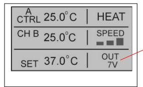
To limit the power on the HCT from ALA, set the voltage output to 7 volts.
