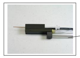
The HCPC can be mounted on a magnetic base with a swivel as pictured above, or via mounting rod (3.2mm 1/8<sup>th</sup> in.) Rods are about 10cm long.
