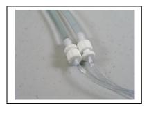
Two Luer fittings shown at left connect the cooler to the HCPC. When the HCPC is to be disconnected, connect the Luer fittings together to form a loop (right) so the fluid does not leak out. When connecting/disconnecting tubes always keep the connections 0.5-1M above the cooler to keep a siphon that will keep the liquid from leaking out during the process.
