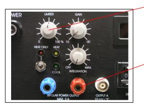
Notice the limiter on the PTC is set with the line at 12 o'clock. This will keep the voltage at just under 7 volts, in the safe zone. The limiter is active whenever the unit is in the control mode. It prevents the PTC from burning out the HCPC when full power is called for.
