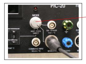
Remember that when the mode switch is set to Direct, DC Voltage will be supplied to the HCPC. The amount will be set by the pin-wheels. The number you set represents a percentage of the full power that can be applied. The Limiter is by-passed in Direct mode, so do not set the value at more than 500, as this represents 50% of 14 Volts, or 7 Volts.
