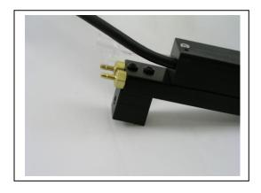
Connect a water supply to these brass fittings for cooling. Minimum flow of 300ml/min. is required for best performance. The perfusion solution should be fed to the clear connector just visible in the background, it is a female Luer fitting, or it can be removed and you can connect directly to the silicone tubing.
