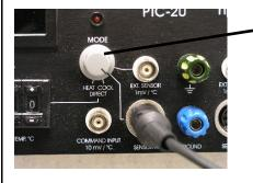
Remember on the npi PTC that when the mode switch is set to Direct, DC Voltage will be supplied to the HCPC. The amount will be set by the pin-wheels. The number you set represents a percentage of the full power that can be applied. The Limiter is by-passed in Direct mode, so for example 500 represents 50% of 14 Volts, or 7 Volts.
