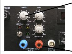
Adjust the limiter on the npi PTC to set the voltage output to max 7 volts. The limiter is active whenever the unit is in the control mode. It prevents the PTC from burning out the HCPC-G when full power is called for. The HCPC-G can handle 12V so the limiter can be turned almost to 100%
