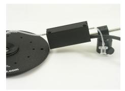
For fluid connection, your HPC-G has a female Luer fitting attached to a short silicone tube.
